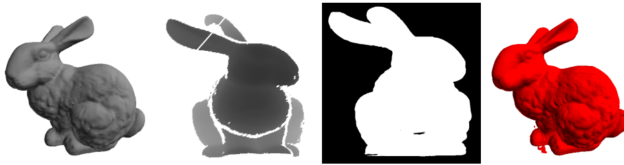
Figure 1: Left to right: Input scan data. Single-scan depth map. All-scans silhouette map. Marching cubes reconstruction using Depth-Augmented Visual Hull.
